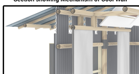
Integrated Piping System with the Hanging Fabric
